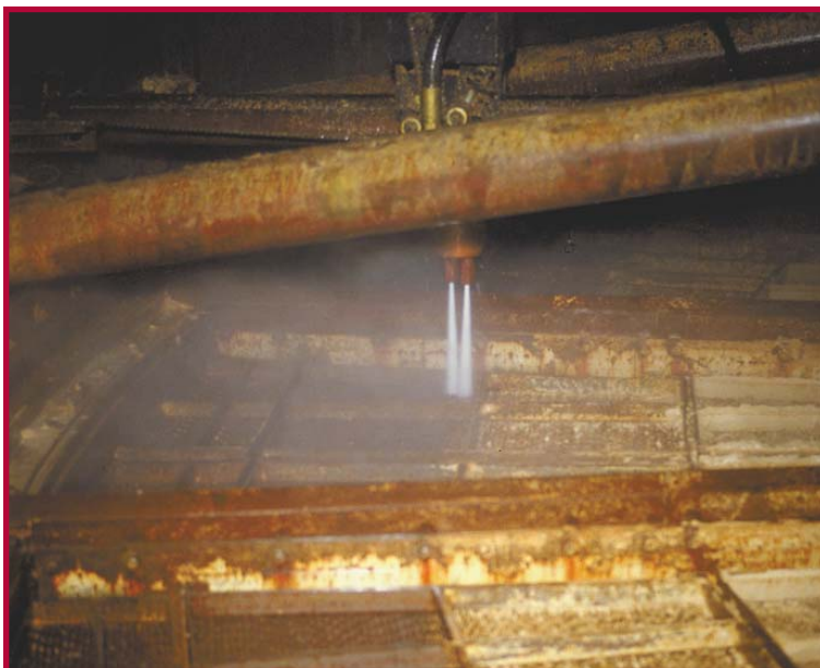
In action, the dark basket portions are freshly clean, the caked, clogged basket portions are pale in color.
