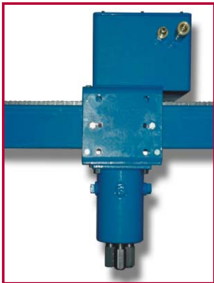
Closeup of a manifold assembly showing how it walks along the mounting bracket. The simple 40 pitch "bicycle style" chain assists in indexing cleaning operation.
